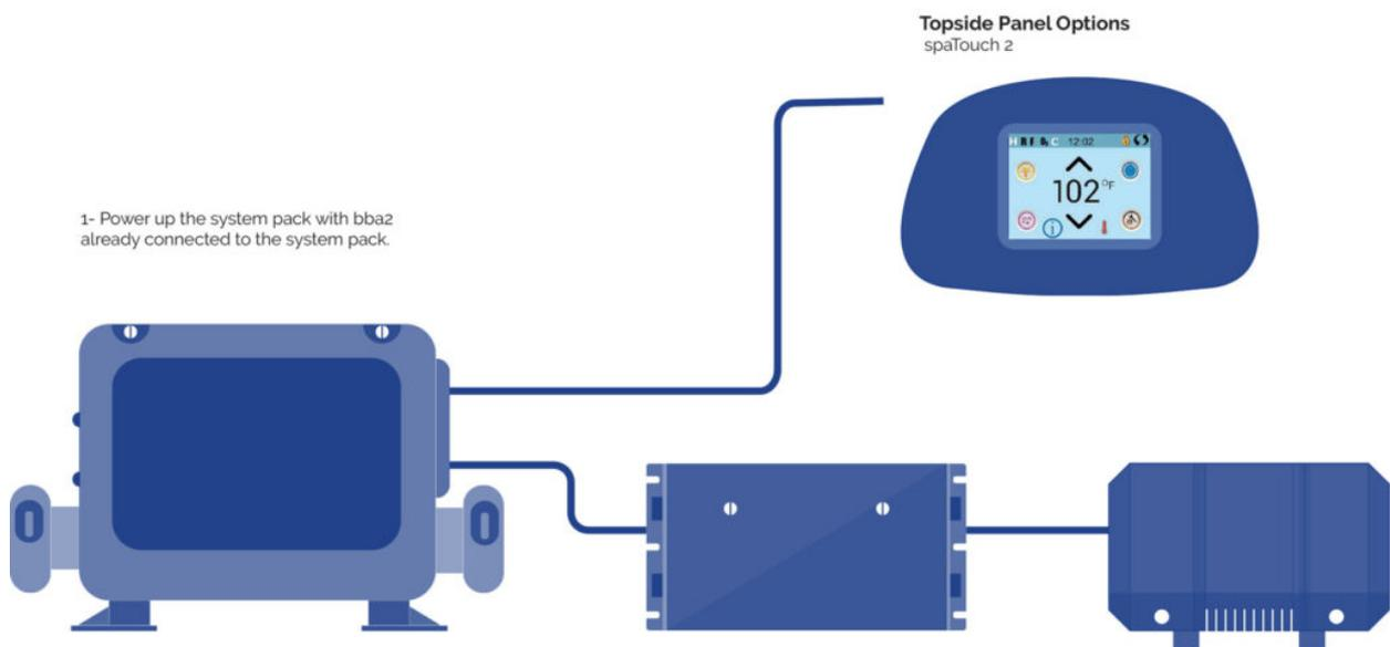
1- Power up the system pack with bba2 already connected to the system pack.
