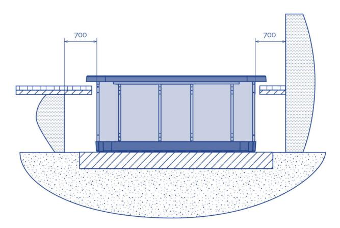
Never fill in the Spa's upper edge with cement or any other material that may have an expansion / contraction different to that of the Spa shell. The Spawould end up cracking.
