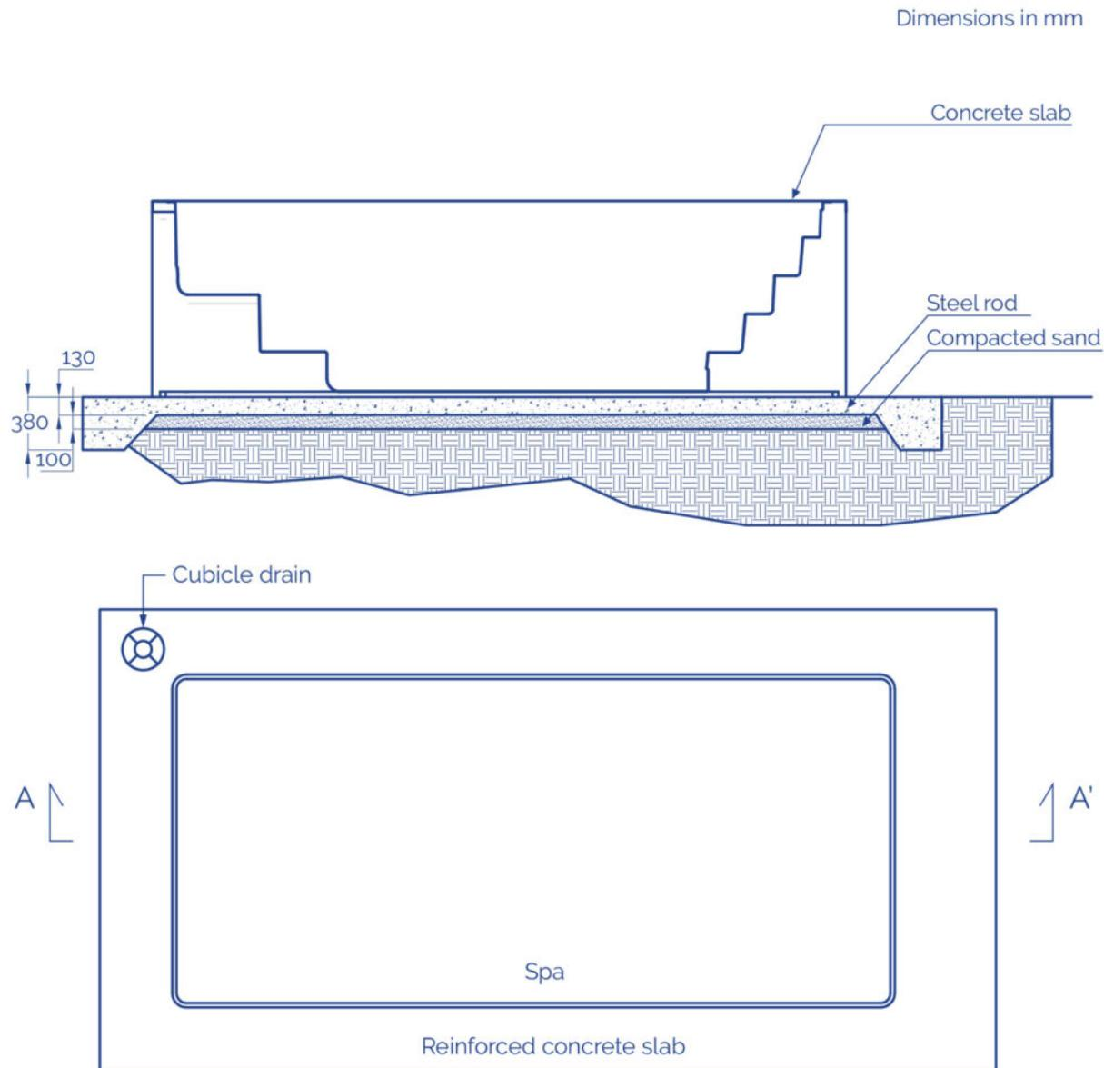
\* Equidistant reinforcement rods in both directions
