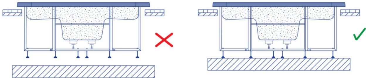
In order to seal the lip of the Spa to the foundations, use elastic silicone special for water installations.
