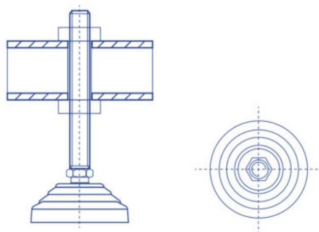
The Spa must be completely supported by the support structure, and must never be supported by its upper edge; otherwise the possible bending would cause the Spa shell to break.
