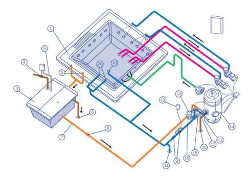
Overflow 1 Overflow drains 2 Balance tank 3 4 Filling solenoid valve Level probes 5 6 Balance tank drain Balance tank suction 7 8 Anti-return valve 9 By-pass valve 10 Drain 11 Spa drainpipe 12 Filter pump Selector valve 13 14 Filter 15 Filter drainpipe 16 Electric Heating 17 Temperature probe 18 Flow detector 19 Ozonator 20 Spa return nozzles
