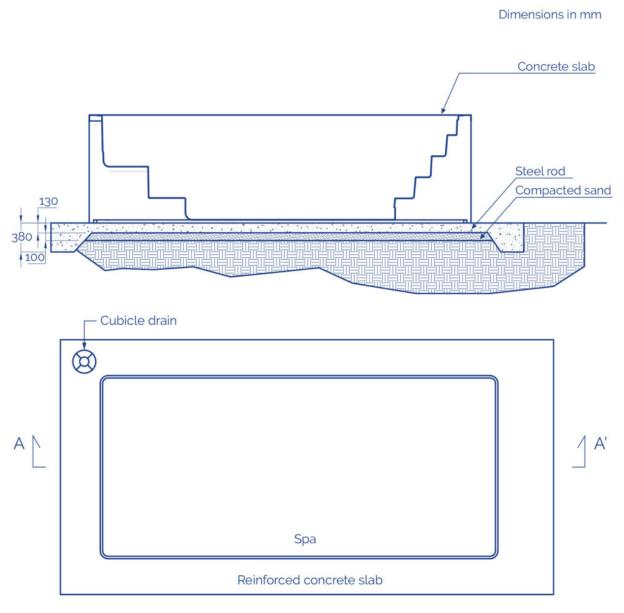
\* Equidistant reinforcement rods in both directions
