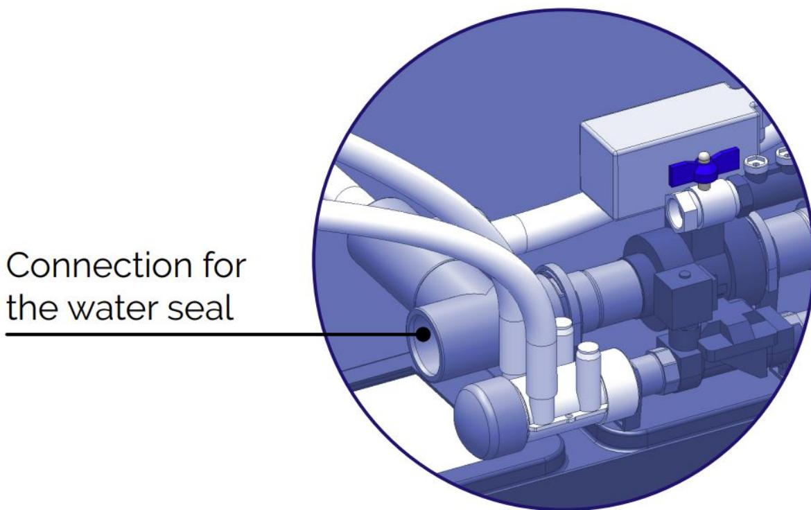
The water seal must be connected via a plain ended PVC pipe that is 50 mm in diameter.
