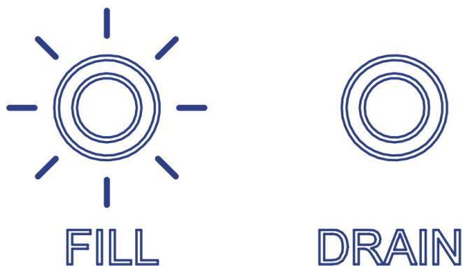
Flashing blue light stabilizes when spa is fully filled.
