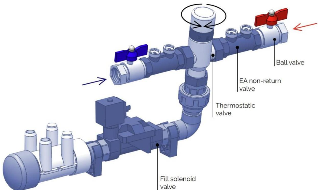
When this is done, the thermostatic valve receives cold water from the network water supply and hot water from the Domestic Hot Water (DHW) system where the hot tub is located. This makes it possible to set the desired temperature at which the hot tub is filled throughout the waterfall.
