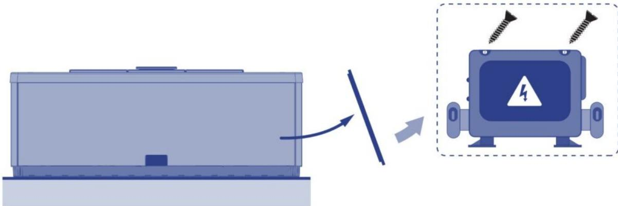
2. Open the control cabinet and connect the spa's electrical panel to the differential.
