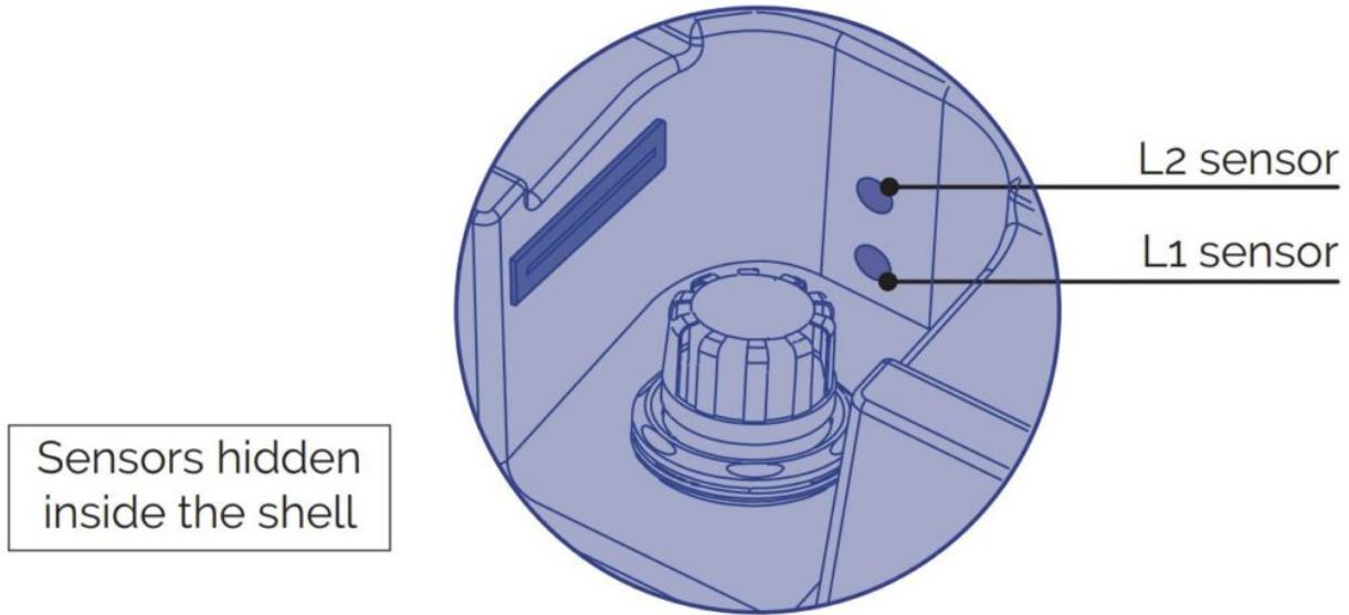
Level L1 is considered safe provided that the sensor detects water for at least 3 consecutive seconds. If water is not detected for that length of time, it remains off, thus activating the automatic filling procedure.
