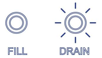
240 minutes later, drain electrovalve will close automatically (OFF mode) and flashing blue light will turn off.
