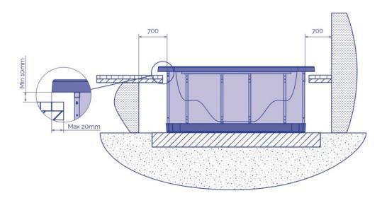
Once settled the Spa, finish the work bearing in mind that the edging of the surface must not be in direct contact with the work (a minimum of 1 cm must be left around the edge).
