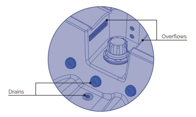
When following a continuous water filling process, the hot tub has an overflow loop composed of two overflows that are located above the height of the telescopic filter. They discharge the excess water into the building's drainage system after it passes through the water seal (not supplied with the spa), regardless of whether the SV is open.
