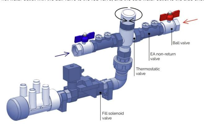
When this is done, the thermostatic valve receives cold water from the network water supply and hot water from the Domestic Hot Water (DHW) system where the hot tub is located. This makes it possible to set the desired temperature at which the hot tub is filled throughout the waterfall.
