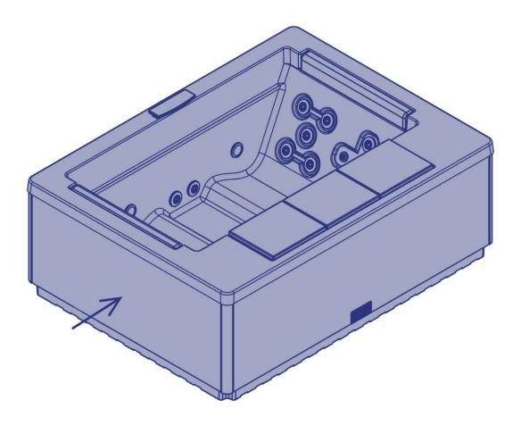
2. Connect the two water supply pipes with a G 3/8" male thread (see the image below). Connect the hot water outlet with the ball valve to the red valve, and the cold water outlet to the blue one.
