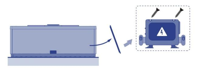
2. Open the control cabinet and connect the spa's electrical panel to the differential.
