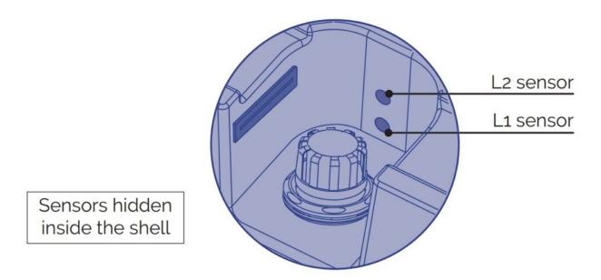
Level L1 is considered safe provided that the sensor detects water for at least 3 consecutive seconds. If water is not detected for that length of time, it remains off, thus activating the automatic filling procedure.
