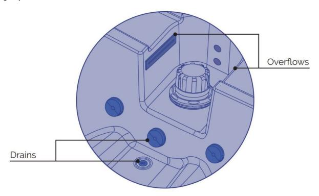
When following a continuous water filling process, the hot tub has an overflow loop composed of two overflows that are located above the height of the telescopic filter. They discharge the excess water into the building's drainage system after it passes through the water seal (not supplied with
