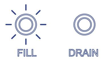
Flashing blue light stabilizes when spa is fully filled.
