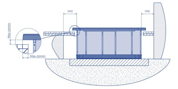
Once settled the Spa, finish the work bearing in mind that the edging of the surface must not be in direct contact with the work (a minimum of 1 cm must be left around the edge).
